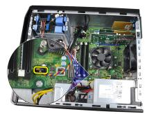
Use a Phillips screwdriver to loosen the captive screws securing the heat sink/fan assembly to the system board.
