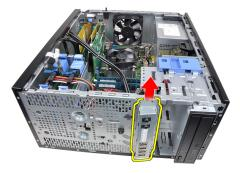
8. Remove the I/O panel by routing the cable through the front of the computer.
