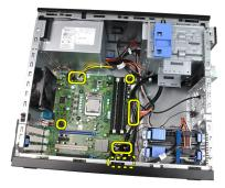
7. Remove the screws that secure the system board to the computer.
