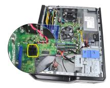
Slide the intrusion switch toward the chassis bottom and remove it from the chassis.
