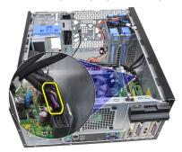
5. Unthread the I/O Panel and FlyWire cable from the clip on the computer.
