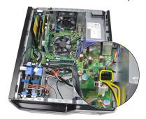
**4.** Pry and remove the system fan away from the four grommets securing it to the back of the computer.
