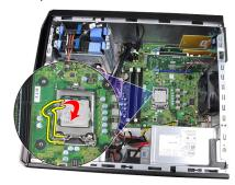
8. Lift the processor to remove it from the socket and place it in antistatic packaging.
