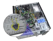
7. Unthread the power switch cable from the chassis clip.
