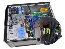
4. Unthread the thermal sensor cable from the chassis clip.
