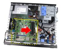
9. Carefully tilt the system board to 45-degrees, and then lift the system board out of the computer.
