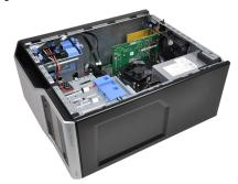
Rotate the bezel away from the computer to release the hooks on the opposite edge of the bezel from the chassis.
