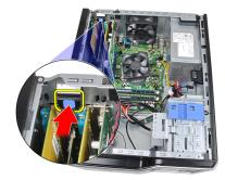
**4.** Gently pull the release lever away from the PCle x16 card until you release the securing tab from the dent in the card. Then, ease the card up and out of its connector and remove it from the system.
