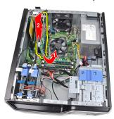
5. Lift the PCIe x1 expansion card (if any) up and out of its connector and remove it from the system.
