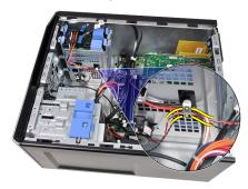
5. Press down the speaker-securing tab and slide the speaker upwards to remove.
