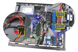
4. Unthread the power cables from the clips in the computer.
