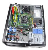
7. Lift the PCI x4 expansion card (if any) up and out of its connector and remove it from the system.
