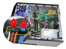
Press both blue securing-bracket tabs inward and lift the hard drive bracket out of the bay.
