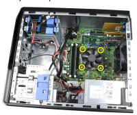
Lift the heat sink/fan assembly upward gently, and remove it from the system. Lay the assembly with the fan facing downward, and with the thermal grease facing upward.
