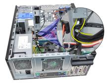
**6.** Remove the screw that secures the I/O panel to the computer.
