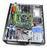
**6.** Lift the PCI expansion card (if any) up and out of its connector and remove it from the system.
