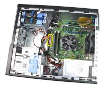
6. Disconnect the 4-pin power cable from the system board.
